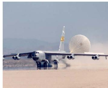
But the B-52 tests revealed that we were far off in our reefed canopy loads. The first 2 B-52 tests showed we were producing first stage loads that would be expected for 27% reefing, whereas we had sized the reefing line to expect 40%. This was a surprise to all involved including Sandia and Knacke, himself. Also the time from disreef to full inflation was much shorter than predicted by conventional methods. So the final reefing line length was resized and verified by continued testing.
